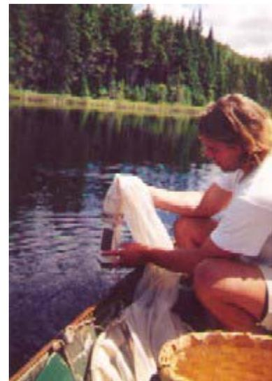
Using Plankton Net to Collect Algae Samples
